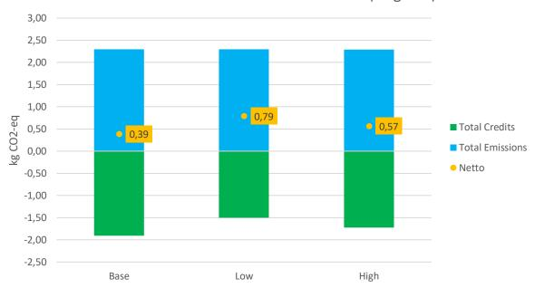
Figure 19 These two graphs illustrate the outcome of using the renewable carbon gas (RCG) for internal electricity production instead of selling the RCG on the market. In the upper figure the cases (base, low and high case) are shown for the waste perspective (1kg MPW processed). In the lower graph the results are shown for the product perspective (1kg R-BTX produced)
