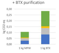
Figure 8 Total global warming impact for the previously mentioned processes and added purification step in kg of CO<sub>2</sub>-equivalents. The left bar represents the waste perspective (1 kg MPW) and the right bar represents the product perspective (1 kg R-BTX). For 1 kg BTX, ~2.68 kg MPW is needed.
