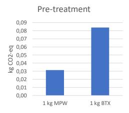
Figure 7 Global warming impact for the pre-treatment step of the process in kg  $CO_2$ -equivalents. The left figure represents the waste perspective (1 kg MPW) and the right figure represents the product perspective (1 kg R-BTX). For 1 kg BTX, ~2.68 kg MPW is needed.
