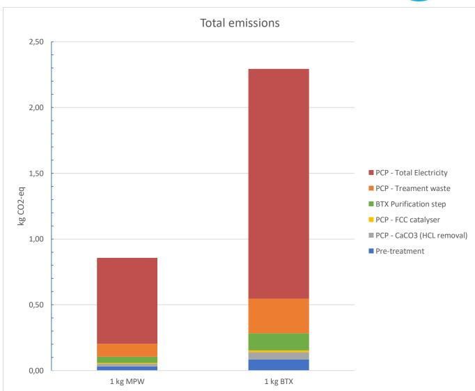
Figure 12 Total impacts of both perspecives in kg of  $CO_2$ -equivalents. The left bar represents the waste perspective (1 kg MPW) and the right bar represents the product perspective (1 kg BTX). For 1 kg R-BTX, ~2.68 kg MPW is needed.
