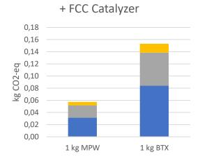
Figure 9 Total impact of the previous processes with added prodution proces of the catalyzer. The left figure represents the waste perspective (1 kg MPW) and the right figure represents the product perspective (1 kg BTX). For 1 kg R-BTX, ~2.68 kg MPW is needed.
