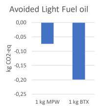
Figure 14 Global warming potential credits for avoided light fuel production in kg of CO2-equivalents. On the left are the credits shown for the waste perspective (1 kg MPW) and on the right for the product perspective (1 kg BTX).
