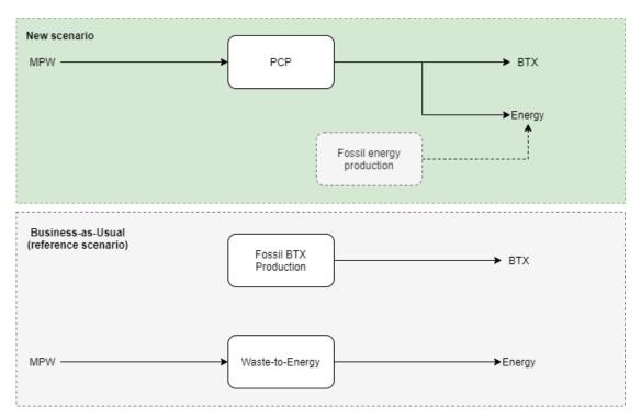
Figure 5 System boundaries for the production of BTX. On the top the PCP process of producing BTX is demonstrated. On the bottom the business-as-usual system for fossil based BTX and the incineration of MPW in a waste-to-energy plant are demonstrated in a high level overview.
