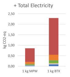
Figure 11 Total impacts of the previous mentioned processes in kg of CO<sub>2</sub>-equivalents. and added the last emission (Total Electricity demand) to the graph. The left bar represents the waste perspective (1 kg MPW) and the right bar represents the product perspective (1 kg BTX). For 1 kg R-BTX, ~2.68 kg MPW is needed.
