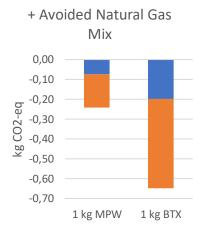
Figure 13 Global warming potential credits for avoided natural gas mix, added to the previous process in kg of CO<sub>2</sub>-equivalents. On the left are the credits shown for the waste perspective (1 kg MPW) and on the right for the product perspective (1 kg BTX).
