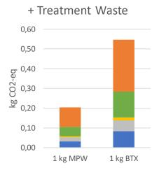
Figure 10 Total imapct of the previous processes and added treatment of waste fractions in kg of CO<sub>2</sub>-equivalents. The left bar represents the waste perspective (1 kg MPW) and the right bar represents the product perspective (1 kg BTX). For 1 kg R-BTX, ~2.68 kg MPW is needed.
