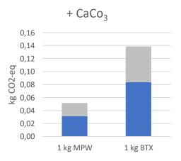
Figure 6 Total impact of the pre-treatment and added production of  $CaCO_3$  in kg  $CO_2$ -eq. The left figure represents the waste perspective (1 kg MPW) and the right figure represents the product perspective (1 kg BTX). For 1 kg R-BTX,  $\sim$ 2.68 kg MPW is needed.
