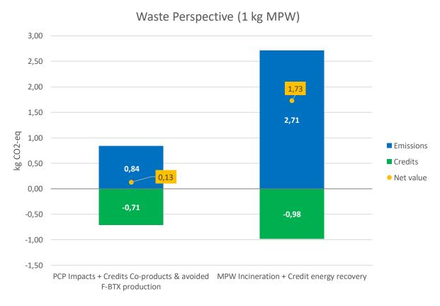
Figure 21 In this graph the results from the PCP management system are compared to the reference MPW incineration as seen from the waste perspective.
