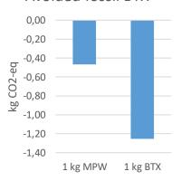
Figure 16 Environmental credits for avoided fossil BTX production for the global warming potential in kg of CO<sub>2</sub>-equivalents. On the left are the credits shown for the waste perspective (1 kg MPW) and on the right for the product perspective (1 kg BTX).
