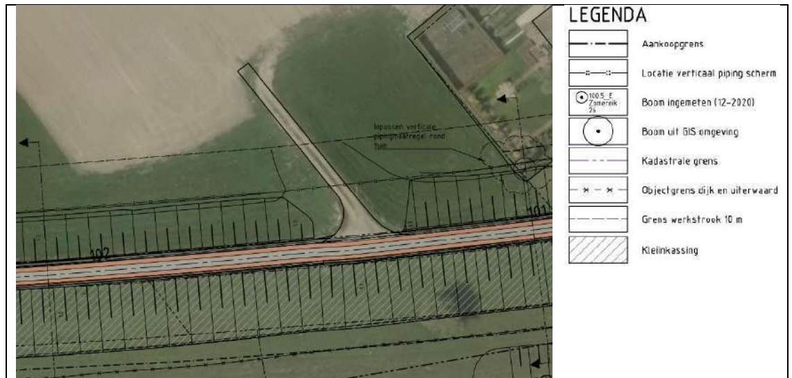
Figuur 15. Inpassing verticale pipingmaatregel dp 101,0 – dp 102,0.
