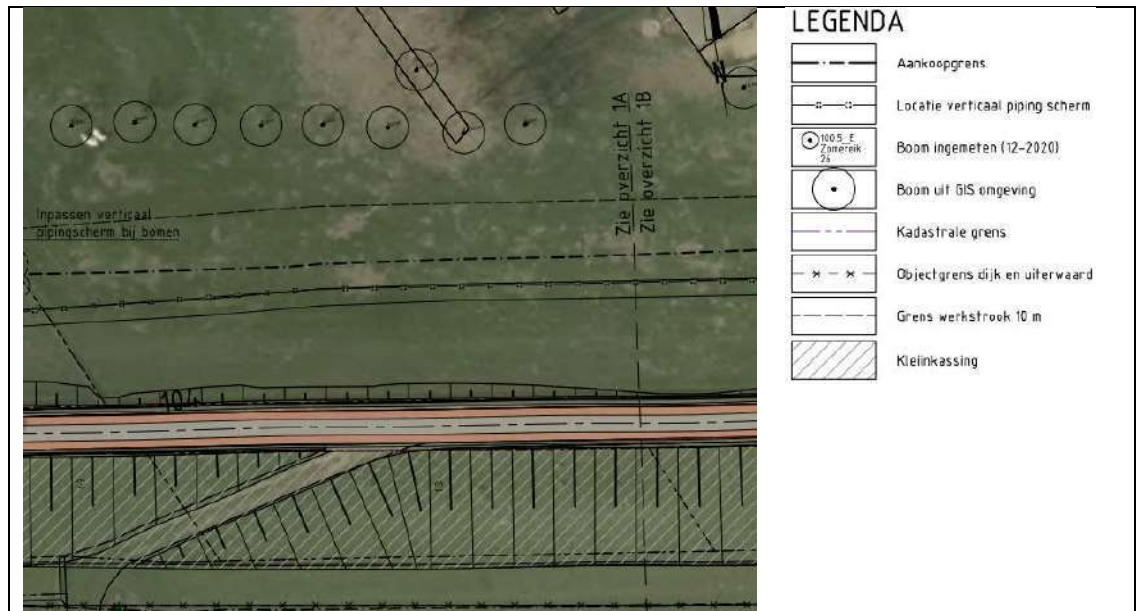
Figuur 17. Inpassing verticale pipingmaatregel dp 103,0 – dp 104,0.
