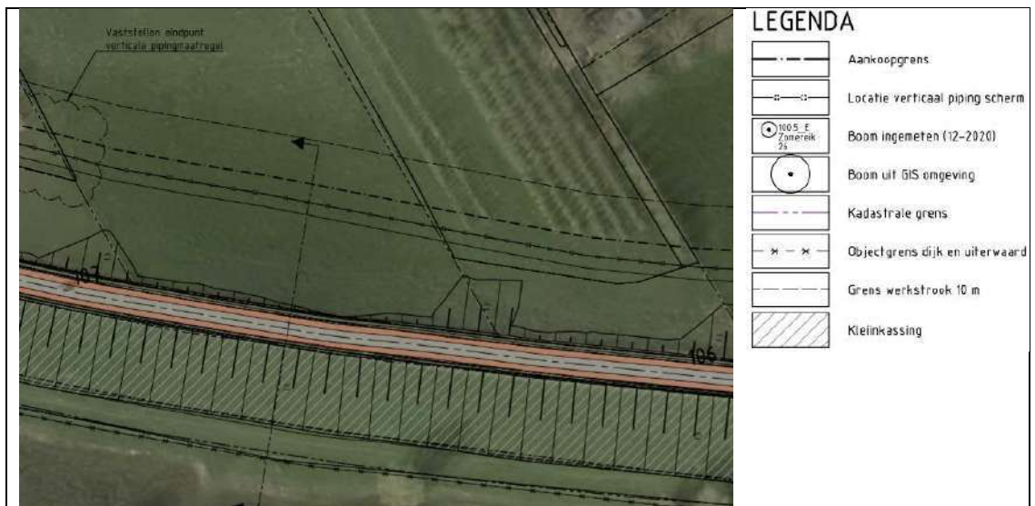
Figuur 20. Inpassing verticale pipingmaatregel dp 106,0 – dp 107,0.
