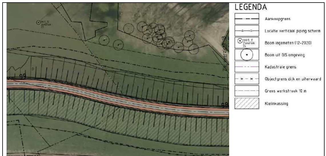
Figuur 12. Inpassing verticale pipingmaatregel dp 98,0 – dp 99,0.
