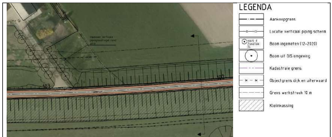
Figuur 16. Inpassing verticale pipingmaatregel dp 102,0 – dp 103,0.
