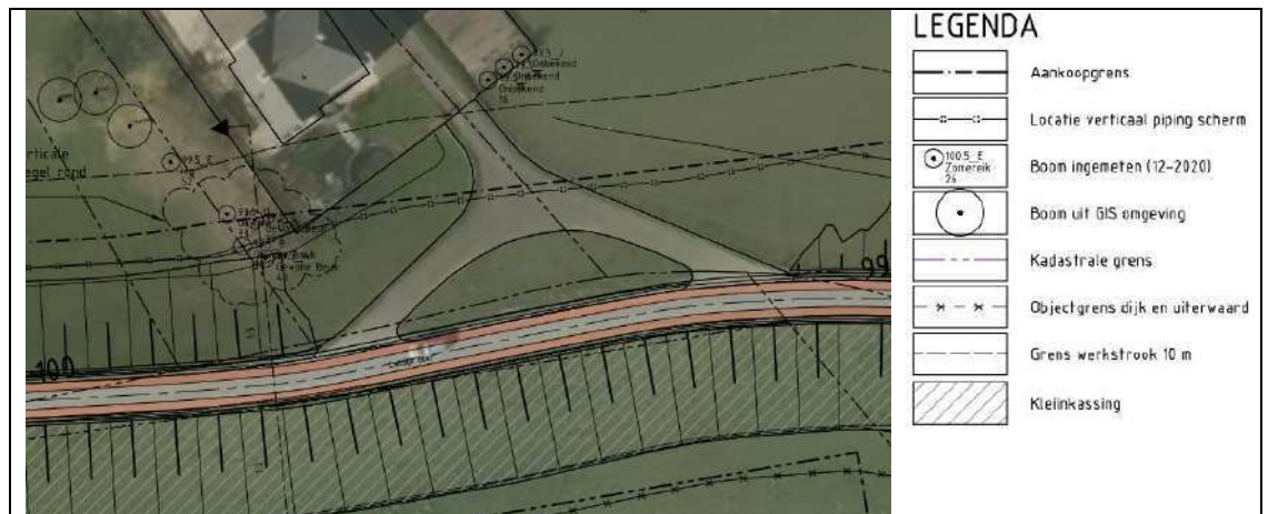
Figuur 13. Inpassing verticale pipingmaatregel dp 99,0 – dp 100,0.
