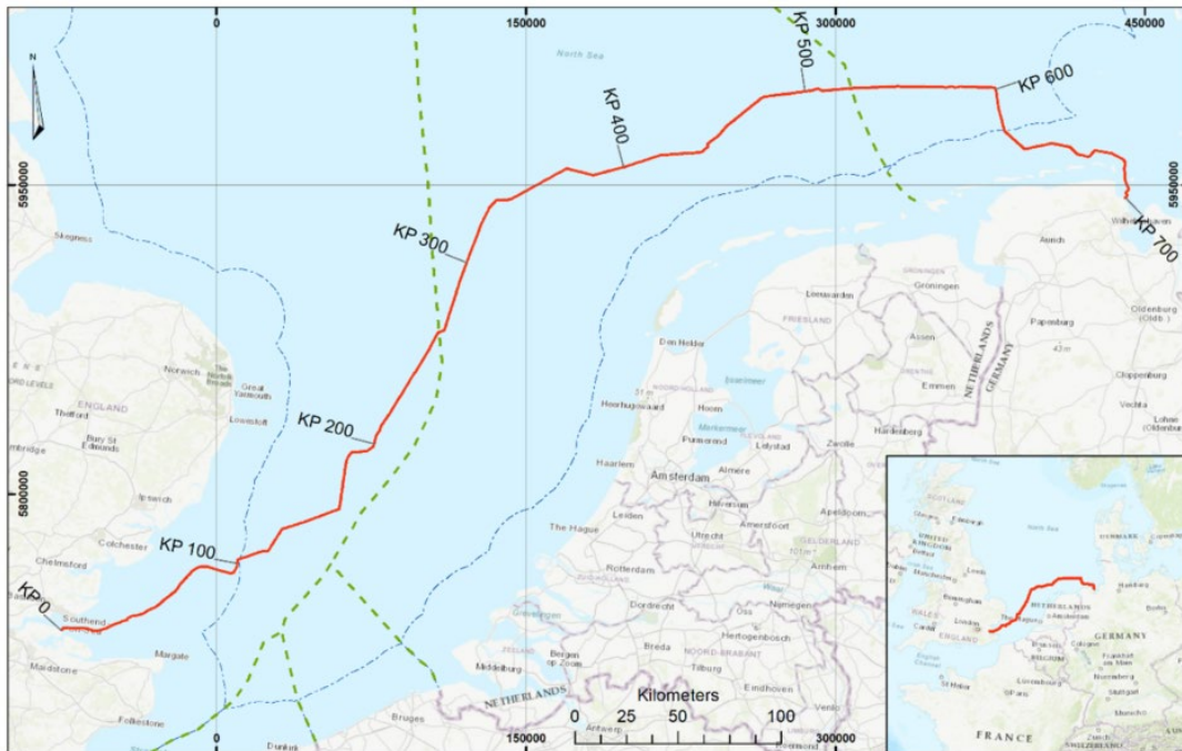
Figure 1: Overview of the planned HVDC submarine cable between Germany and the UK with the section of the Netherlands EEZ (red line = cable route; dashed green line = EEZ borders; dotted blue line = territorial borders).
