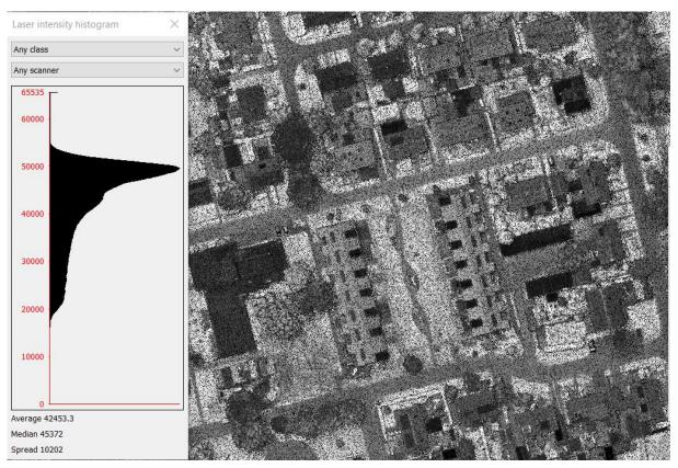
Figure 10: Image shows intensity values in top view with histogram
