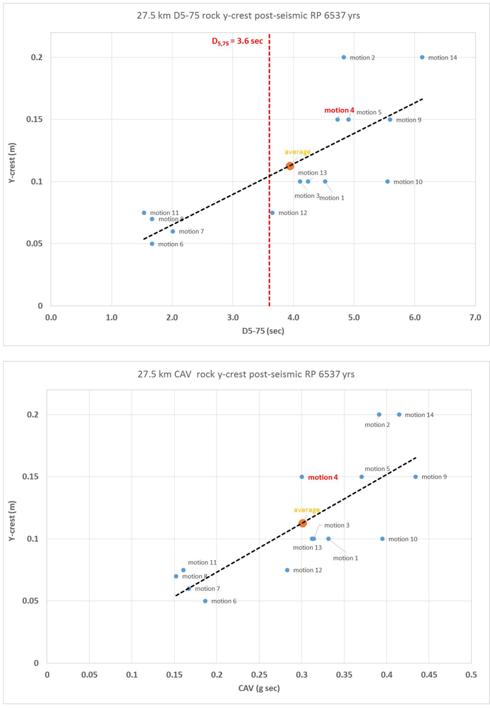
Figure 42. Range of crest settlements versus significant duration (upper illustration) and cumulative absolute velocity (lower illustration) from 14 different ground motions for Delfzijl Design Basis Case (Deltares 2017).
