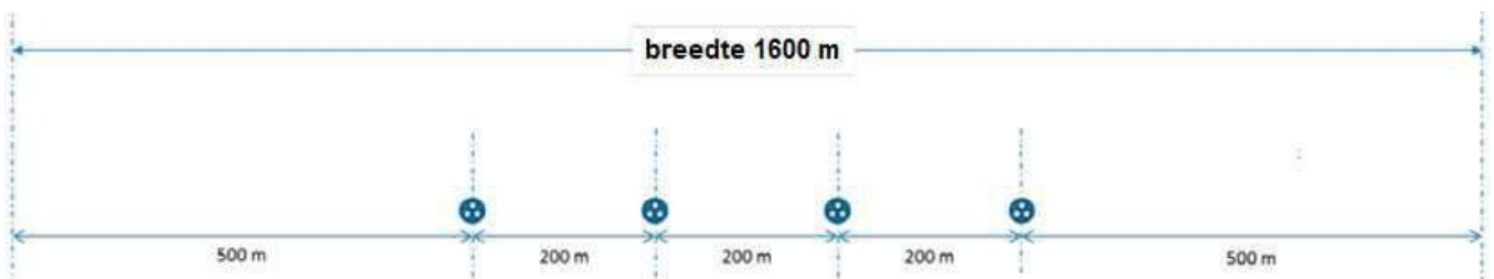
Figure 33 Cable corridor offshore section - 4 cable systems
