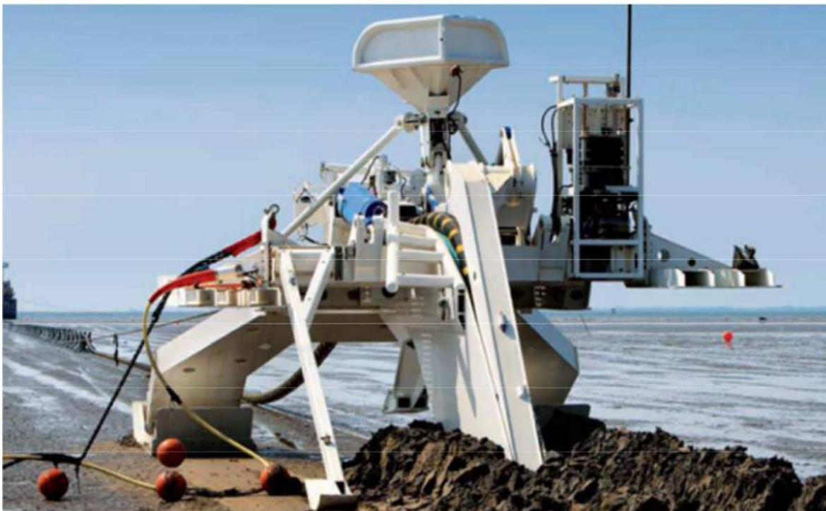
Figure 42 Sea Stallion cable plough
