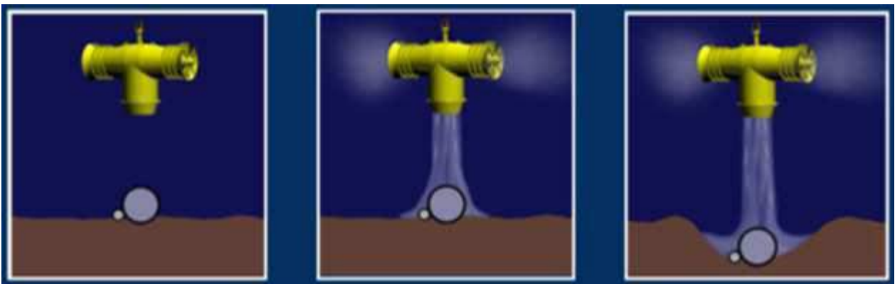
Figure 43 Mass flow excavation
