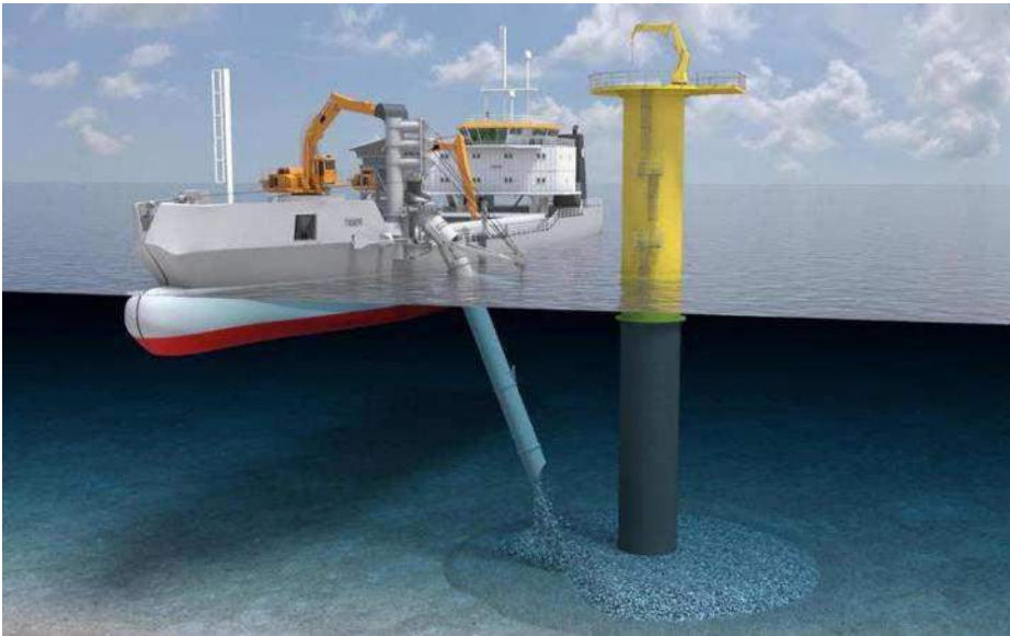
Figure 57 Rock installation vessel
