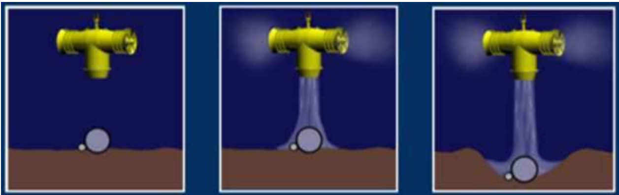
Figure 43 Mass flow excavation
