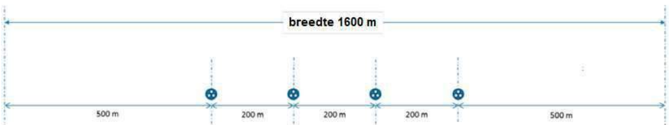
Figure 33 Cable corridor offshore section - 4 cable systems
