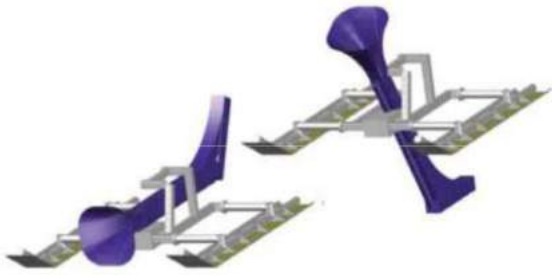
Figure 37 Typical Jet sledge
