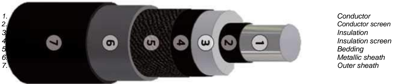
Figure 6 Typical HVAC 220 kV land export cable
