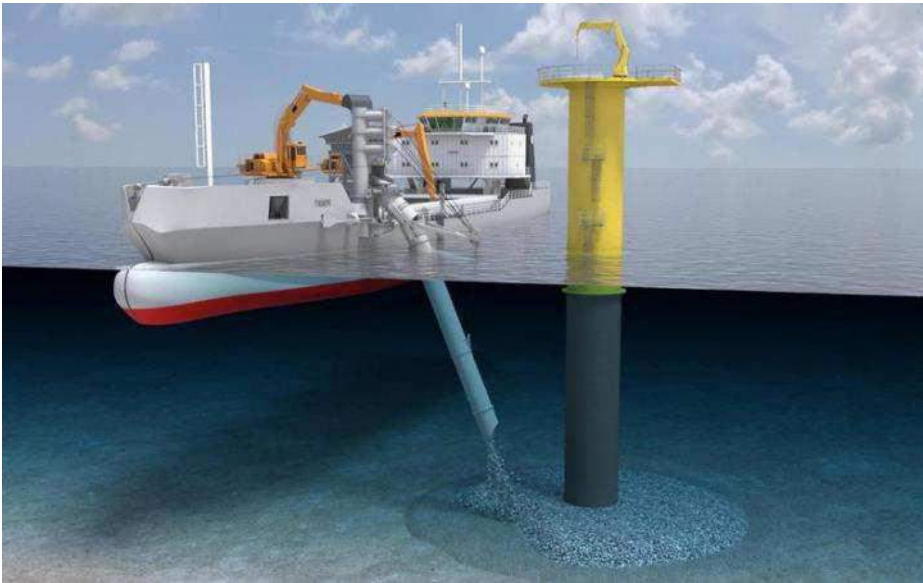
Figure 57 Rock installation vessel
