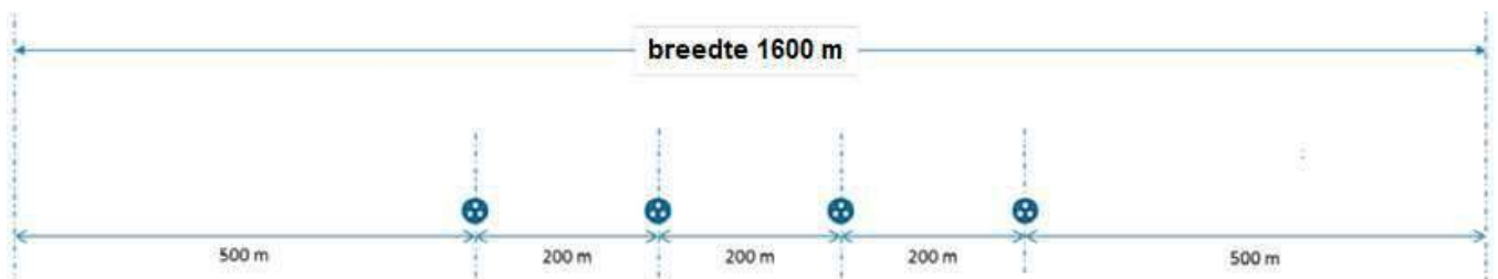
Figure 33 Cable corridor offshore section - 4 cable systems
