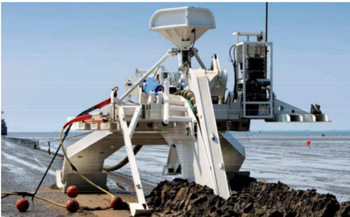
Figure 42 Sea Stallion cable plough
