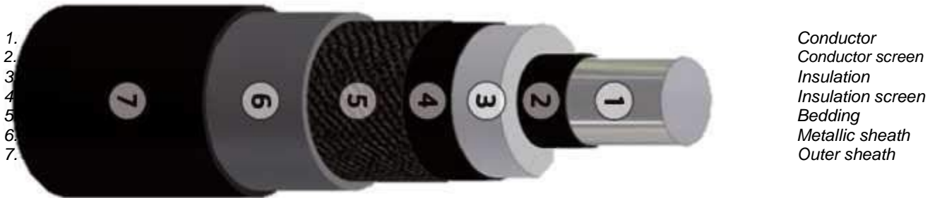
Figure 6 Typical HVAC 220 kV land export cable
