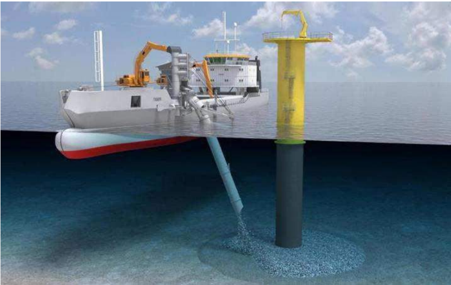
Figure 57 Rock installation vessel
