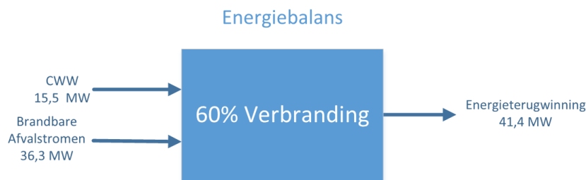
Figuur 8.2: Energiebalans non-submerged combustion (variant P1)
