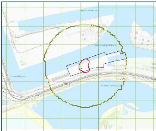
Figuur B3.3: PR één opslagtank (20.000 m 3 ) in tankput TP03
