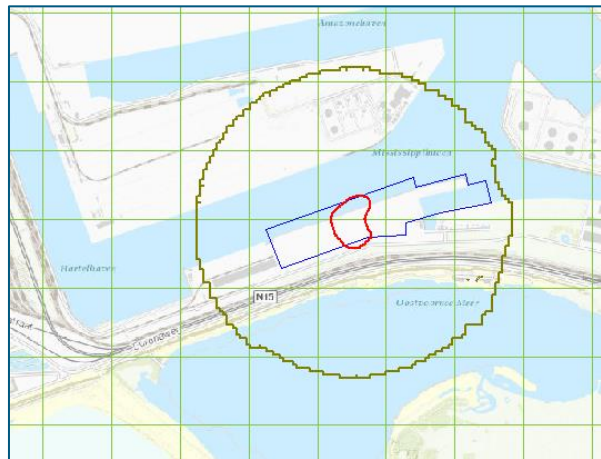
Figuur B3.4: PR één opslagtank (20.000 m 3 ) in tankput TP04
