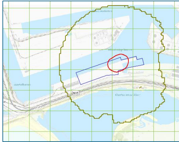
Figuur B3.8: PR één opslagtank (35.000 m3) in tankput TP08
