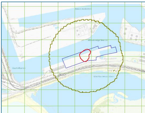
Figuur B3.5: PR één opslagtank (20.000 m 3 ) in tankput TP05
