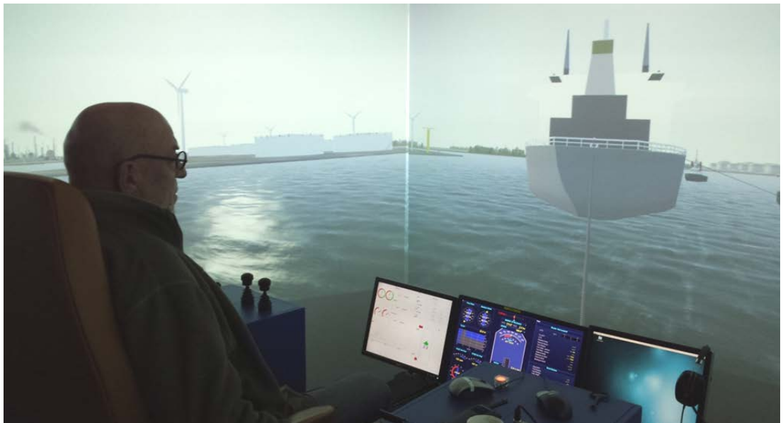
Figure 4-2 View of tug master steering the stern tug on the tug simulator
