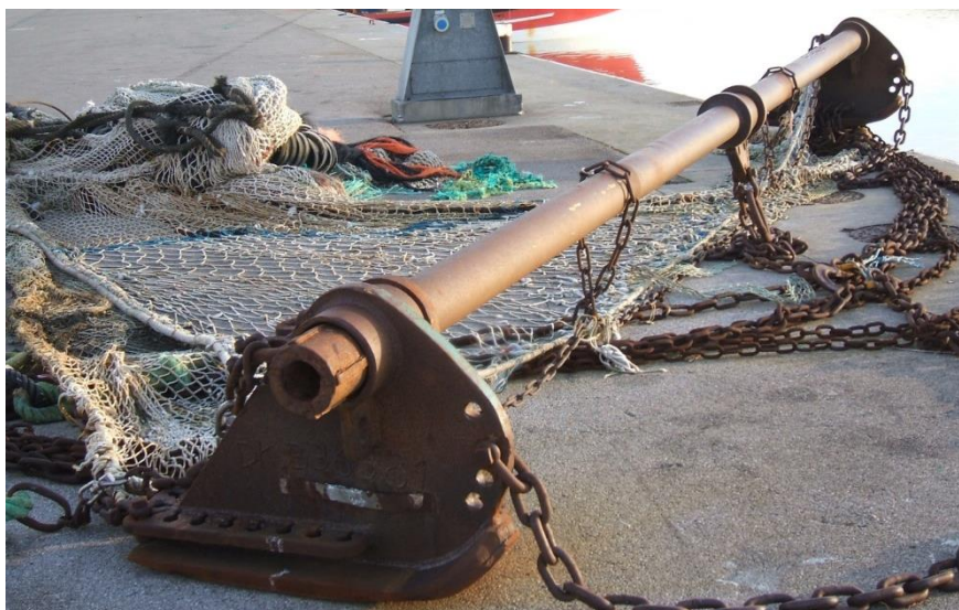
Figure 20. 10-metre Open Beam Trawl Rig with "Tickler" Chains
