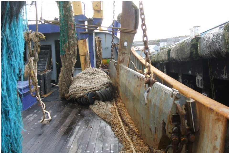
Figure 21. Sumwing Beam on board Belgian Beam Trawler
