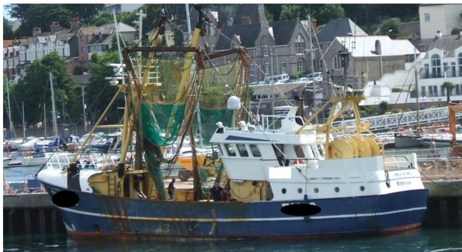
Figure 17. Typical 22 metre, 300hp Euro-cutter Shrimp Beam Trawler
