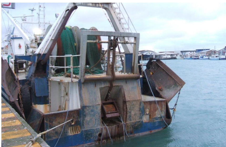
Figure 19. Twin-Rig Trawl Boards and Centre Roller Assembly on board Danish Shrimp Trawler
