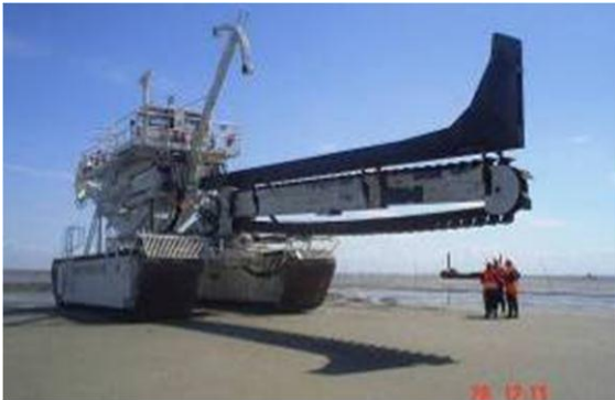
Figure 22: Typical self-supporting cable trencher
