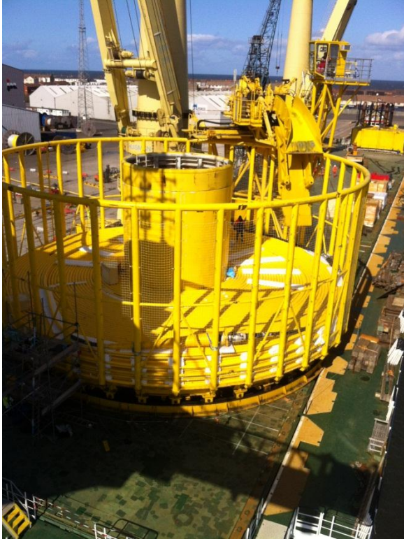
Figure 3: Turntable on board of transport ship
