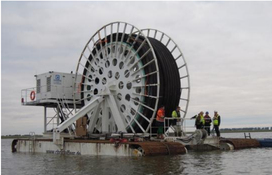
Figure 27: Modular transport vehicle with cable drum
