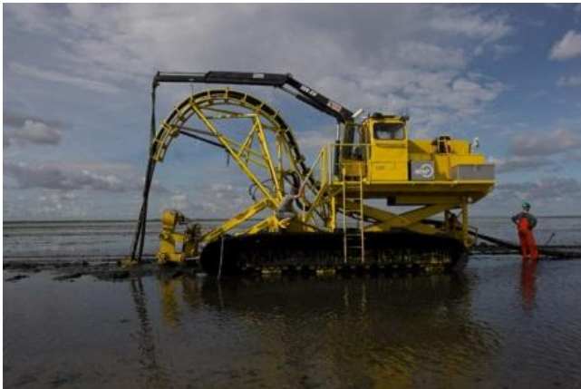
Figure 23: Typical self-supporting vibration plough
