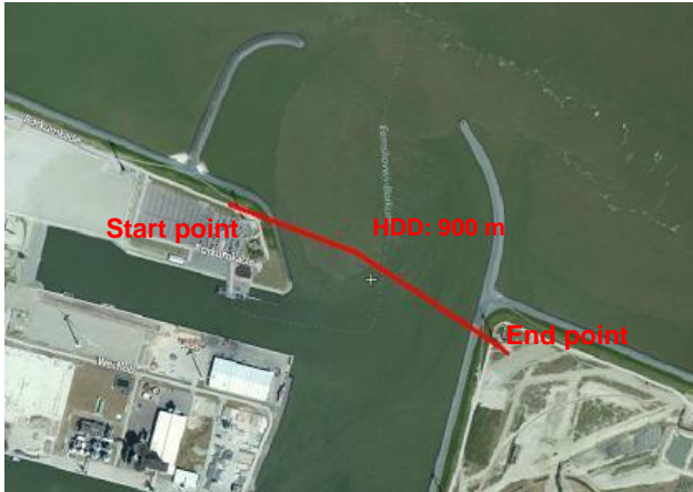
Figure 17: HDD drilling route (red line) Doekgat (Eemshaven)
