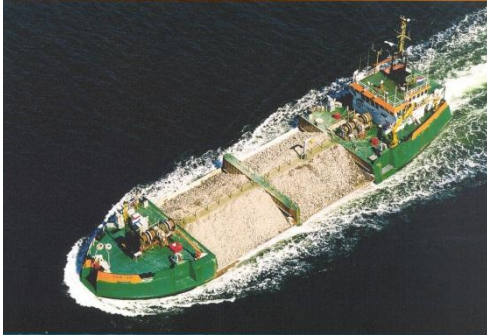
Figure 50: Typical example of a side stone dumper
