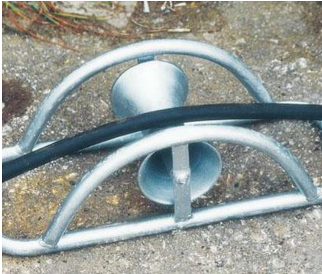
Figure 7: Typical cable roller
